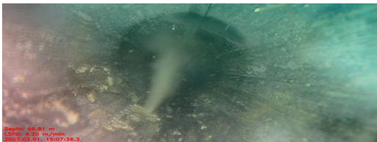
Figure 10—Figure indicates camera run snapshot identifying leak at depth 66 m MD RKB
