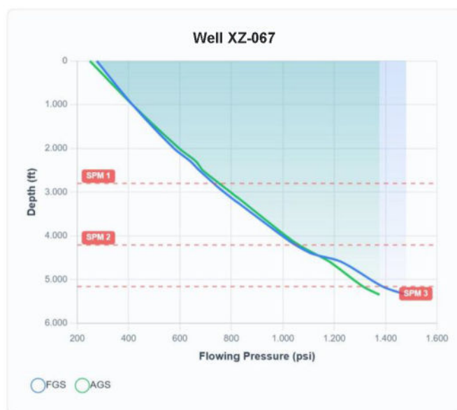
Figure 6—A graph for well XZ-067, showing a close match between the AGS and FGS pressure profile
