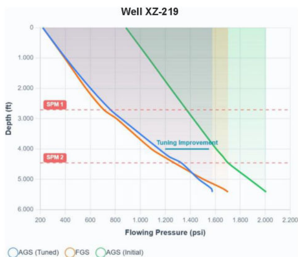
Figure 5—A graph of Flowing Pressure vs. True Vertical Depth for well XZ-219, plotting the AGS calculated profile against the FGS measured profile.
