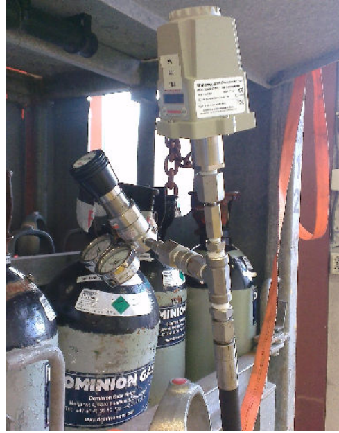
Figure 4.2: Nitrogen tank and a regulator, used to inject gas and regulate the pressure in the hoses.
