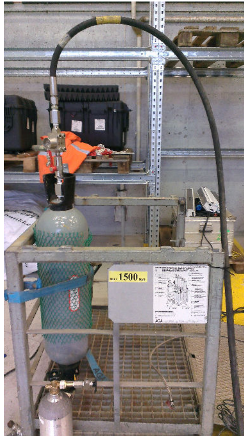
Figure 4.10: Gas bottle used as chamber for the acoustic gun
