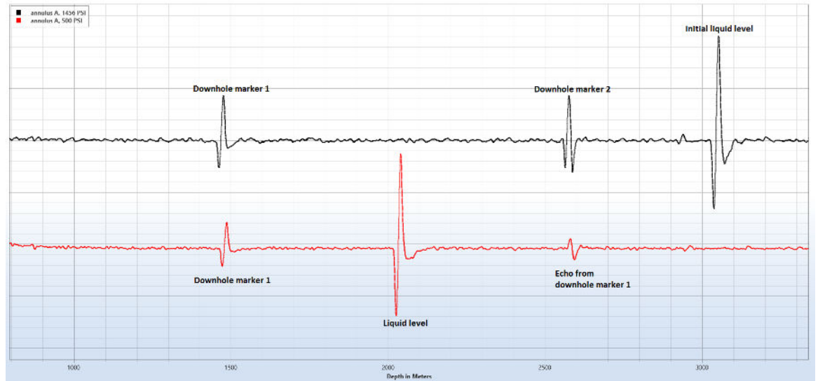
Figure 1.2: Example of an acoustic signal which also reveals a severe leak
