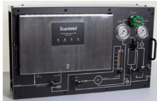
Figure 4—Shkorin Gas Analyser (SGA)
